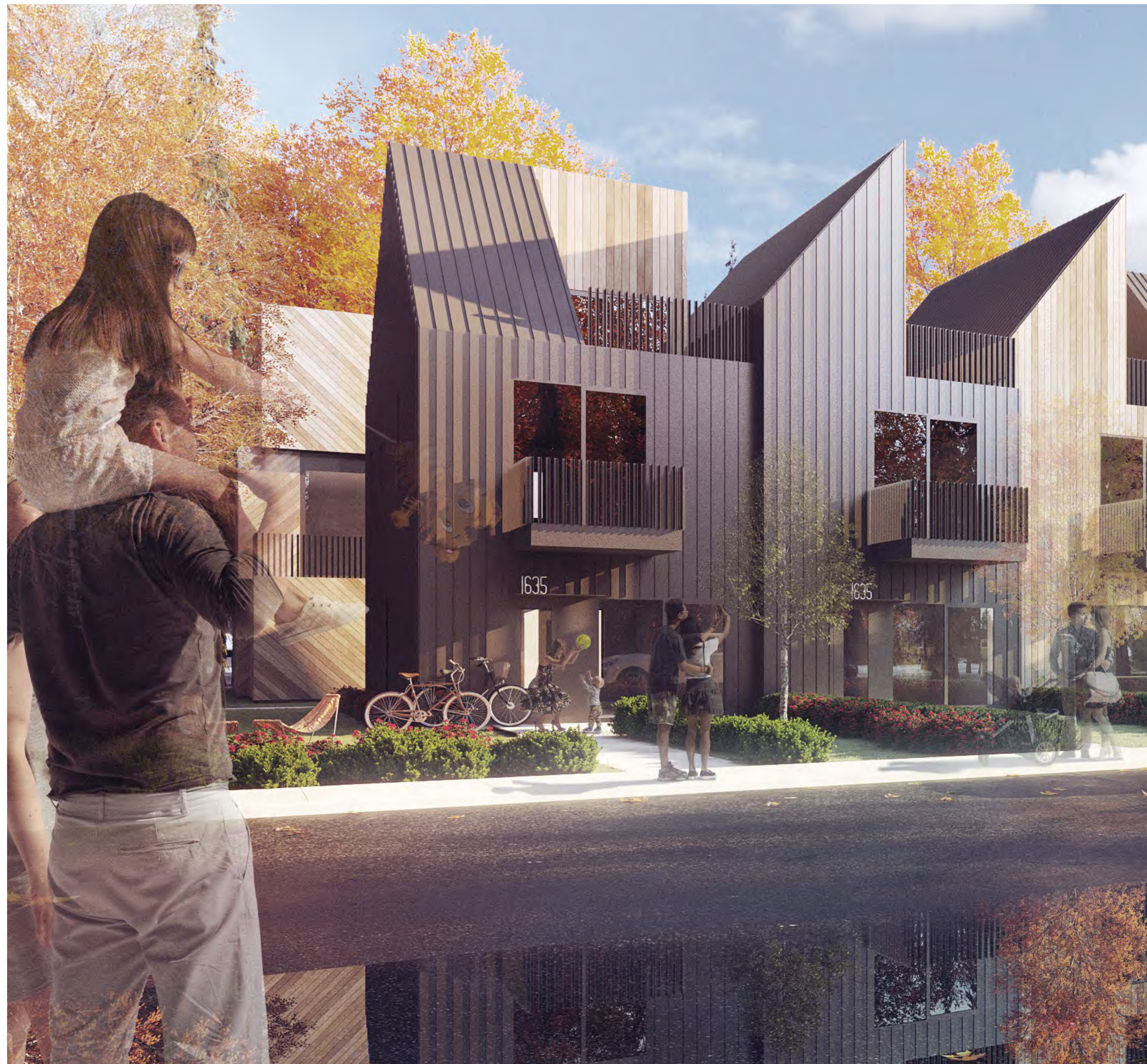
Metal standing seam roof & wall cladding in neutral dark tones
